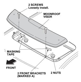
13. Install two screws through the two side brackets; then loosely install the nuts as shown. Remove the masking tape.
