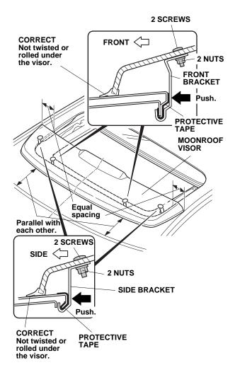
15. Tighten the two screws and two nuts on the front of the visor first, then tighten the two screws and two nuts on the sides. Tighten while applying pressure so that there is no gap between the roof panel and the brackets. Torque the screws to 2 N·m (1.5 lbf·ft). 16. Remove the IMPORTANT INFORMATION label and the shop towels.
